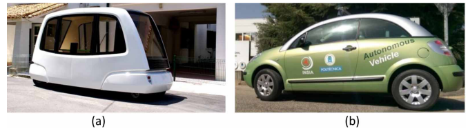
Fig. 1. Some connected autonomous vehicles to be tested in the Lisbon Pilot. Shuttle vehicles, as in (a), will be used in urban-node scenario, while instrumented and autonomous vehicles, like the one in (b), will be deployed in motorway scenarios.
